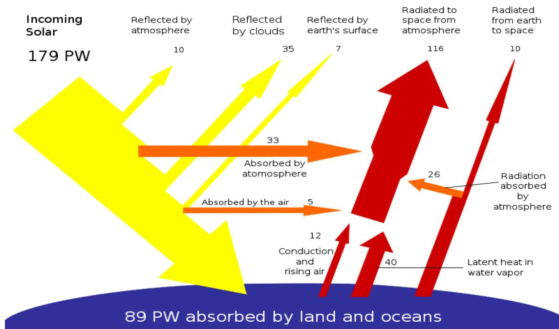
**Fig. 8.** Solar incidence and reemission with very many thanks to the original Authors. (Kim, 2018) (Original source not known)
